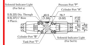
Single Solenoid: Spring Offset DSG-01-2B\*-A\*-70/7090
